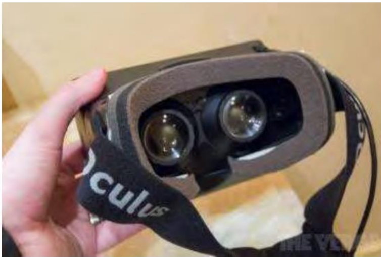
Figure 2.15 The Rift is a binocular HMD intended for immersive computer games. It is under development by Oculus, which was acquired by Facebook in 2014 for 2B$. This large acquisition has raised the interest in HMD technology world-wide.
