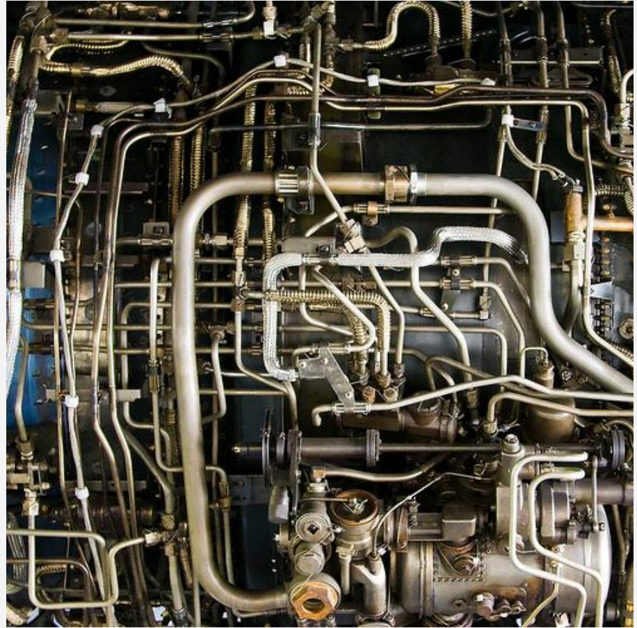
A small section of the pipework on a Pratt and Whitney J58 turbojet engine. © Fragments of Eternity
