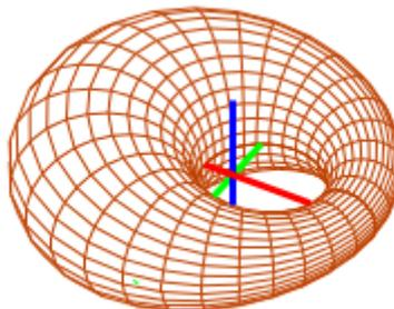
Fig. 9: Cyclide as 4 rational Bézier patches.
