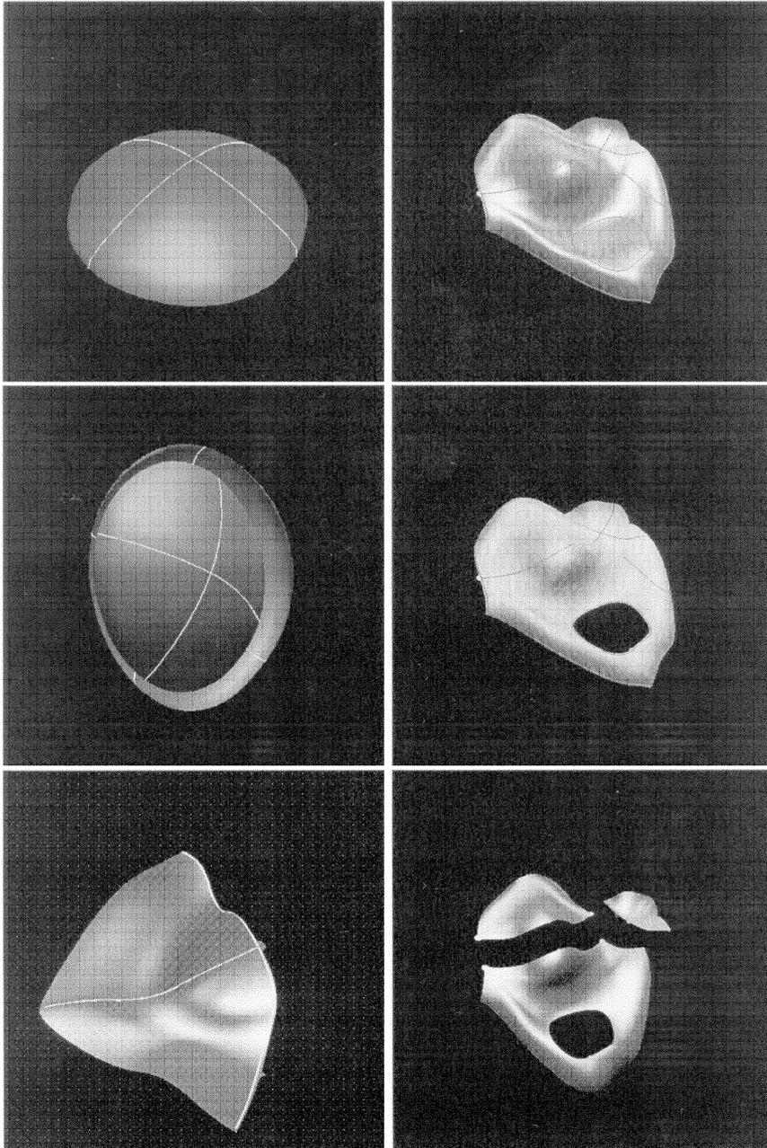
Fig. 15. Left: Color shaded pictures of the surfaces in Fig. 12 interpolating intersecting curves on the interior (top and middle) and on the boundary Fig. 11. Right: Trimming of a subdivision surface along interpolated curves. Surface of Fig. 12 (top) trimmed along the interior closed curve (middle), and then split into 3 pieces (bottom).
