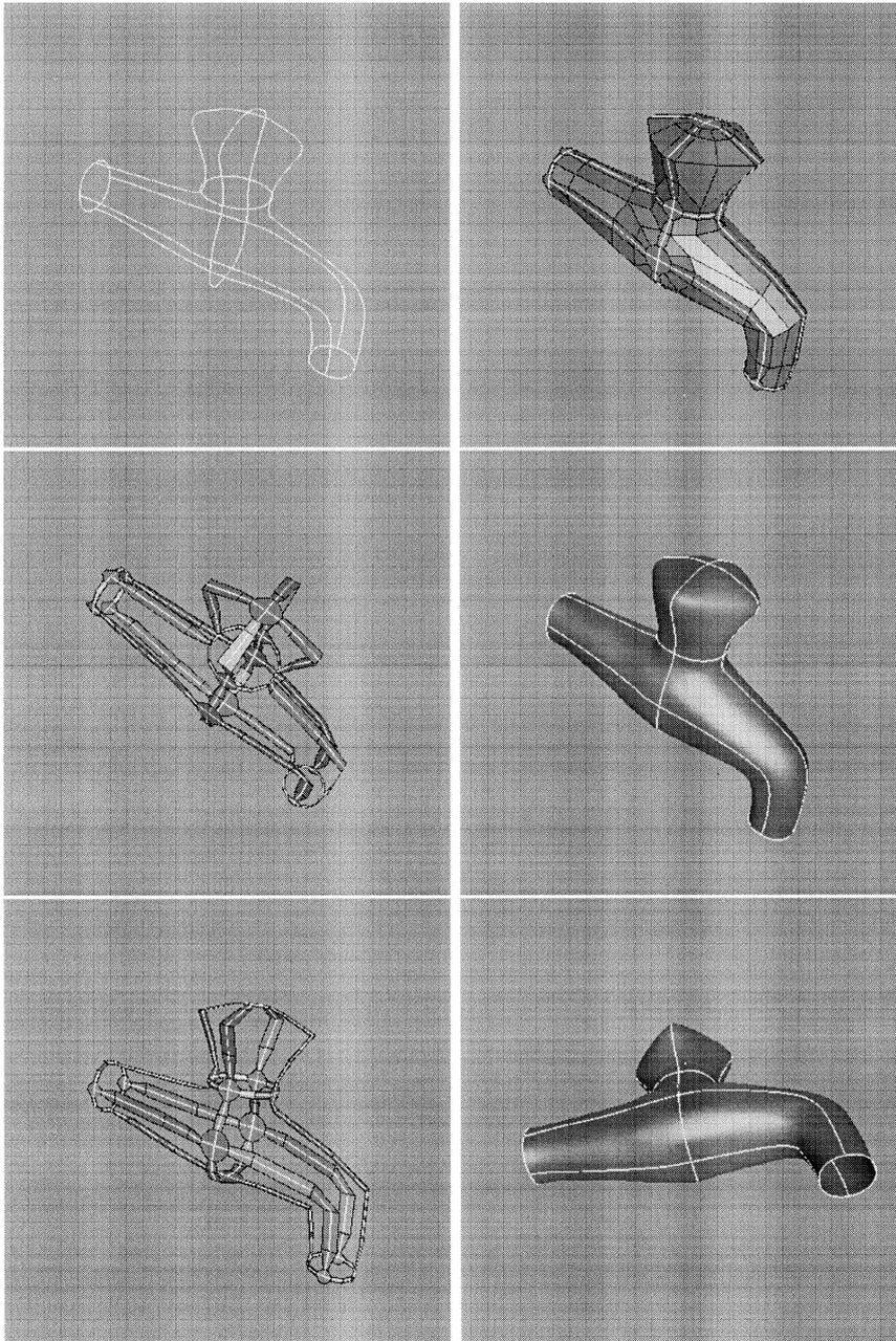
Fig. 13. A tap surface interpolating an arbitrary mesh of curves with various  $n$ -sided ( $n = 3, 4, 5$ ) regions. Left column from top: A mesh of given curves and two views of the polygonal complexes defining these curves. Right column from top: A network incorporating these complexes and two views of the corresponding limit surface interpolating the given curves.
