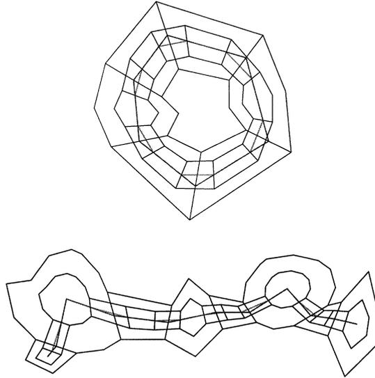
Fig. 7. Invariance of a symmetric polygonal complex under Doo–Sabin: Annular case (top), strip case (bottom).
