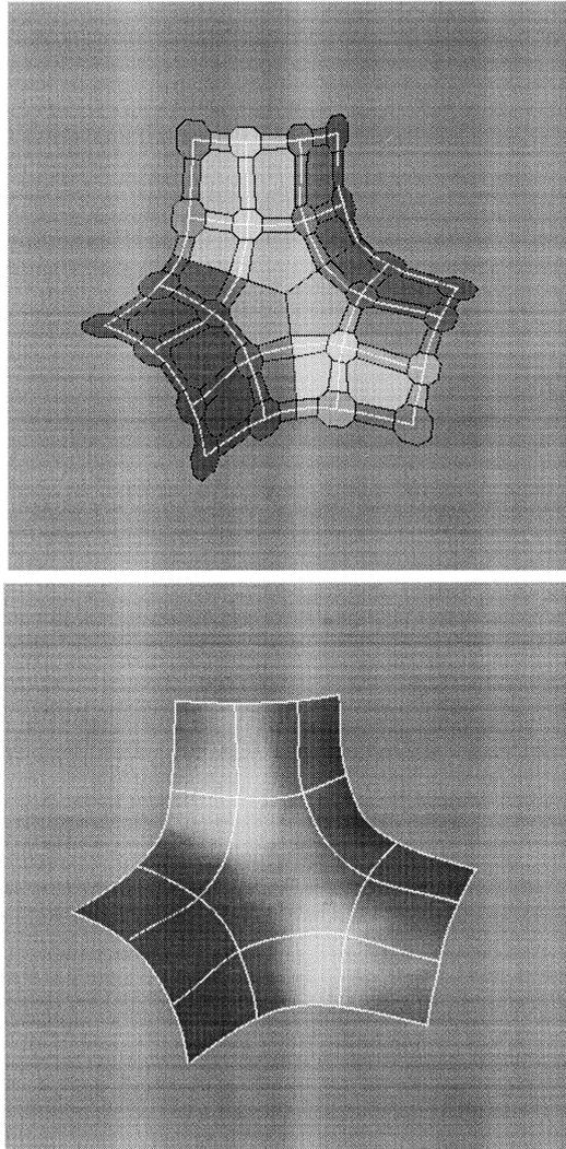
Fig. 14. A surface interpolating a mesh of curve with a 6-sided region enclosed by these curves: A polyhedron with polygonal complexes (top) and limit surface interpolating the predefined curves (bottom).
