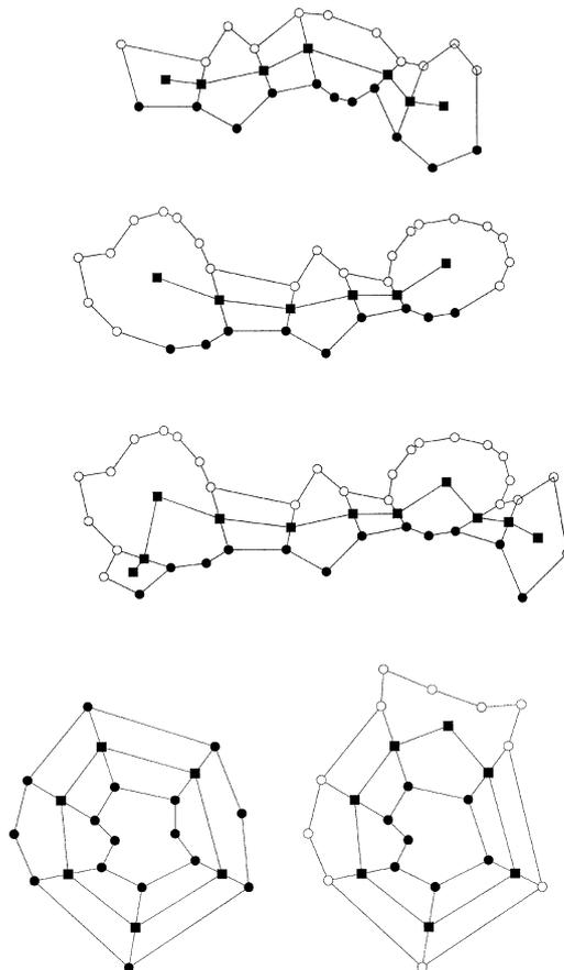
Fig. 5. Various symmetric polygonal complexes and their mid-polygons: Starting from top: a strip whose panels are all single-reflected, a strip with double-reflected end-panels, a general form of a strip complex, an annular complex with single-reflected panels (left), and an annular complex with one double-reflected (right) are shown with original vertices (solid circles), reflected vertices (hollow circles), and mid-polygons vertices (solid squares).
