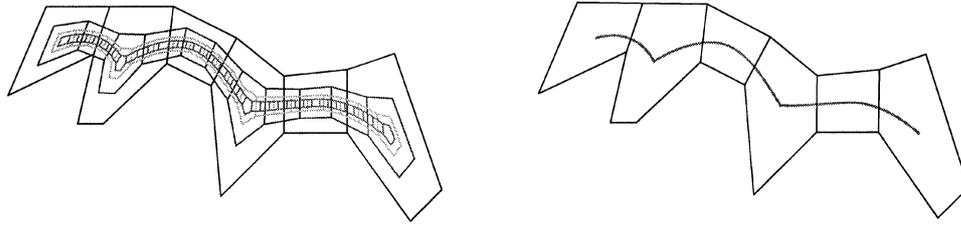
Fig. 3. Convergence of non symmetric polygonal complexes. Three successive subdivisions (left) and the limit curve (right) are shown. Note that  $G^1$  is not achieved at the  $n$ -sided non symmetric face.
