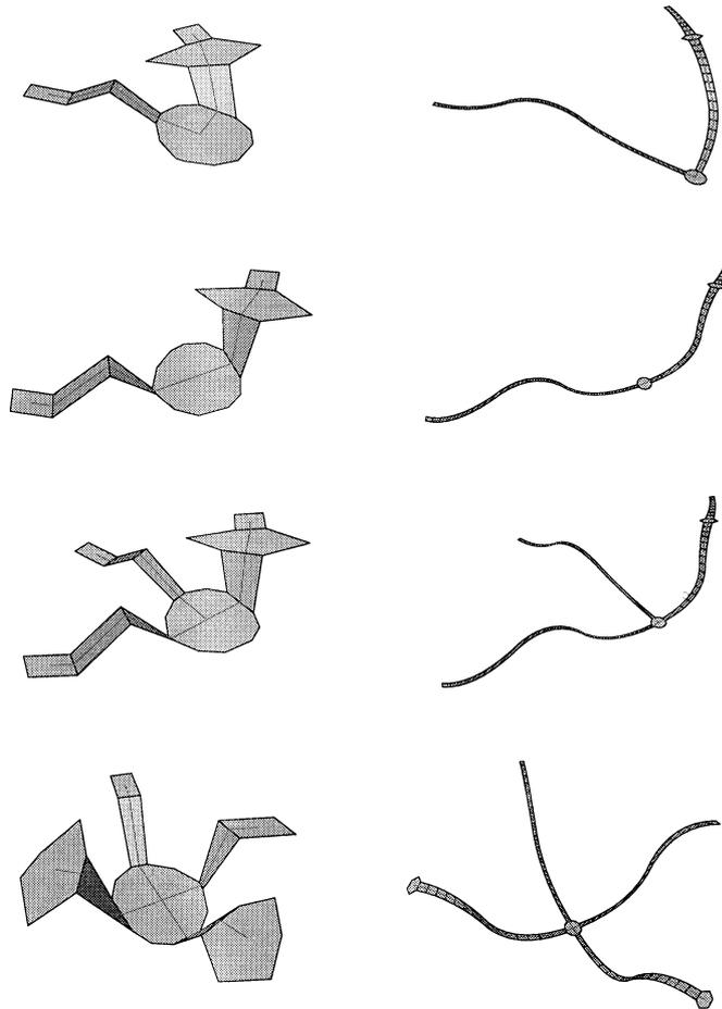
Fig. 9. Convergence of polygonal complexes sharing one double-reflected panel. From top: two complexes giving two limit curves with  $C^0$  joint, two complexes giving two limit curves with  $C^1$  joint, three complexes giving three limit curves, and four complexes giving four limit curves. In all figures, complexes and mid-polygons arc shown on left, their third subdivisions and limit curves are shown on right.
