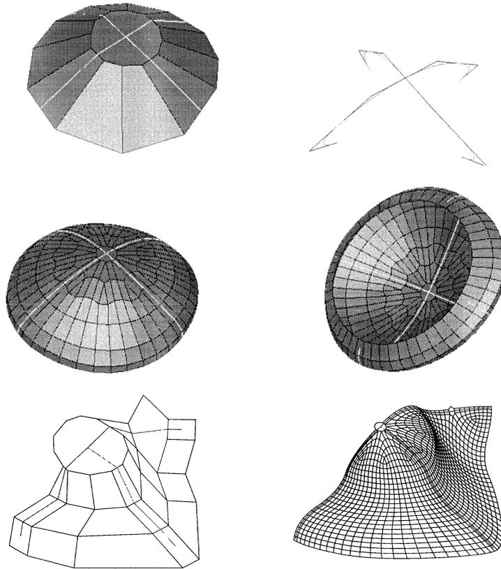
Fig. 11. Interpolating intersecting curves: A surface network containing four strip complexes and their mid-polygons (top left), the limit curves and their polygons (top right), two views of the corresponding limit surface (middle), another surface network containing two strip complexes (one boundary and one interior) and their mid-polygons (bottom left), and the corresponding limit surface (bottom right).
