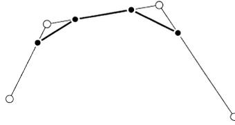
Fig. 1. A control polygon (hollow vertices) and its first Chaikin's subdivision (solid vertices).
