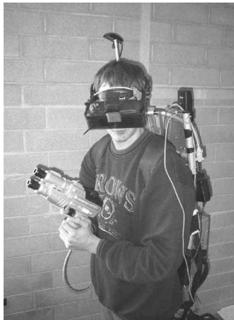
Figure 1.6: The ARQuake player. With HMD, haptic gun, backpack with computer and head tracker. Figure is taken from [123].
