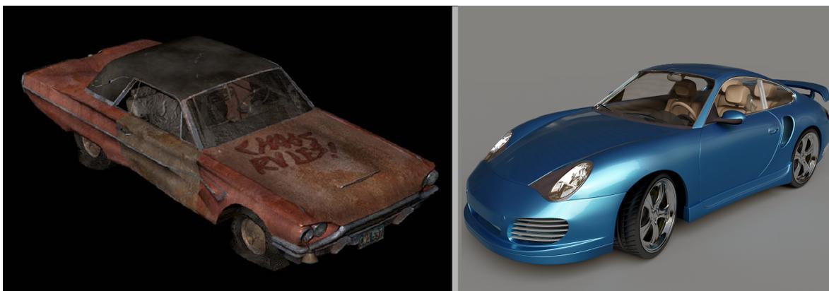
**Figure 1.1:** A comparison of old and new car coat. Left: Rough surface of rusty car absorbs and scatters incident light [27]. Right: Smooth polished coating of new car reflects light source [68].
