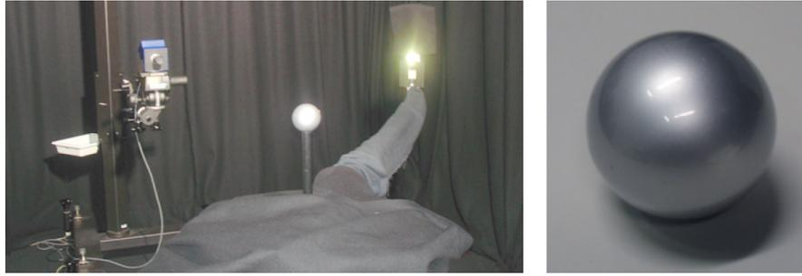
**Figure 4.1:** *Left: A photograph of BRDF measurement system. Right: The measurement target, a sphere painted with car paint [30].*
