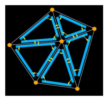
As you can see in the diagram, the half-edges that border a face form a circular linked list around its perimeter. This list can either be oriented clockwise or counter-clockwise around the face just as long as the same convention is used throughout. Each of the half-edges in the loop stores a pointer to the face it borders (not shown in the diagram), the vertex at its end point (also not shown) and a pointer to its pair. It might look something like this in C:
